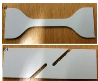
Fig. 3 (a) Tensile dogbone specimen and (b) proposed shear specimen (without notch)
