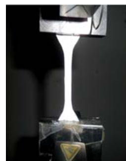
Fig. 5 Tensile testing of PP
