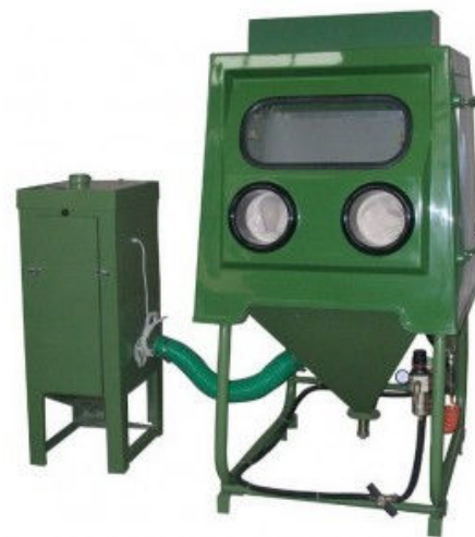
Fig. 1 Experimental set-up for sand blasting process [10]
