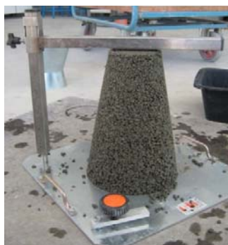
Fig. 5 Consistency of fresh concrete
