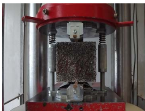
Fig. 3 Splitting tensile test
