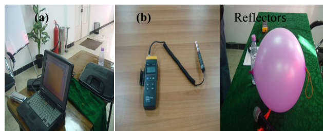
Fig. 1 Materials used for experiment, (a): PC and Spectra software, (b): Sound level meter Lutron SL-4013, (c) balloon
