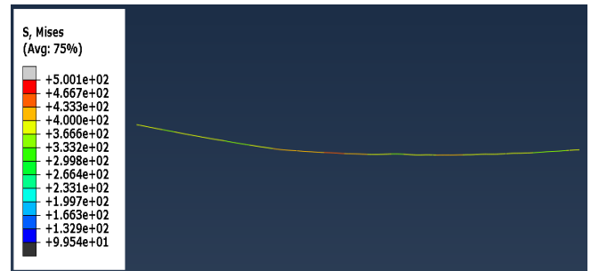
Fig. 7 Stress distribution for cable wire (case2)
