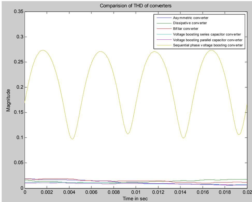
Fig. 21 Total Harmonic Distortion with Low Pass Filter
