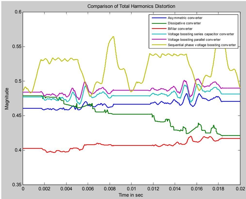
Fig. 13 Total Harmonic Distortion without Harmonic Reduction Techniques
