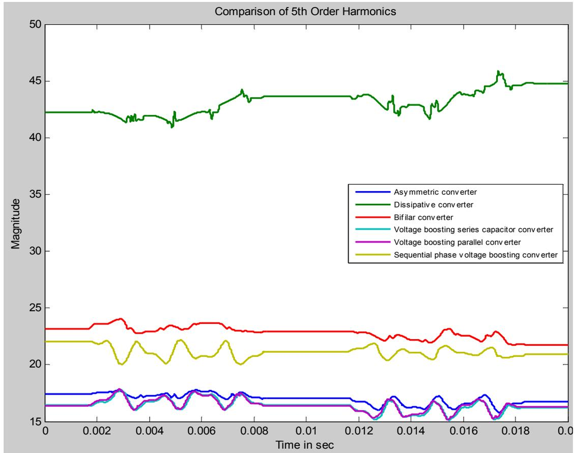
Fig. 10 5<sup>th</sup> Order Harmonics without Harmonic Reduction Techniques
