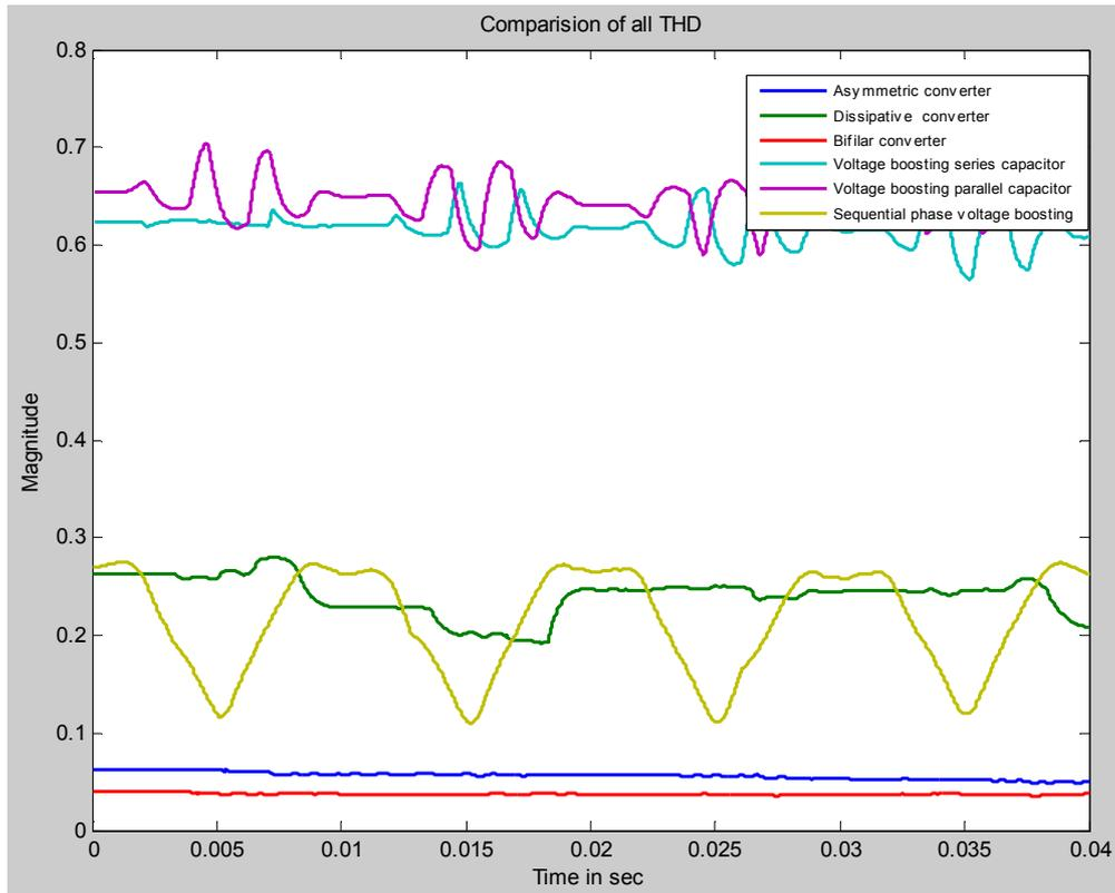
Fig. 17 Total Harmonic Distortion with Star Delta Transformer
