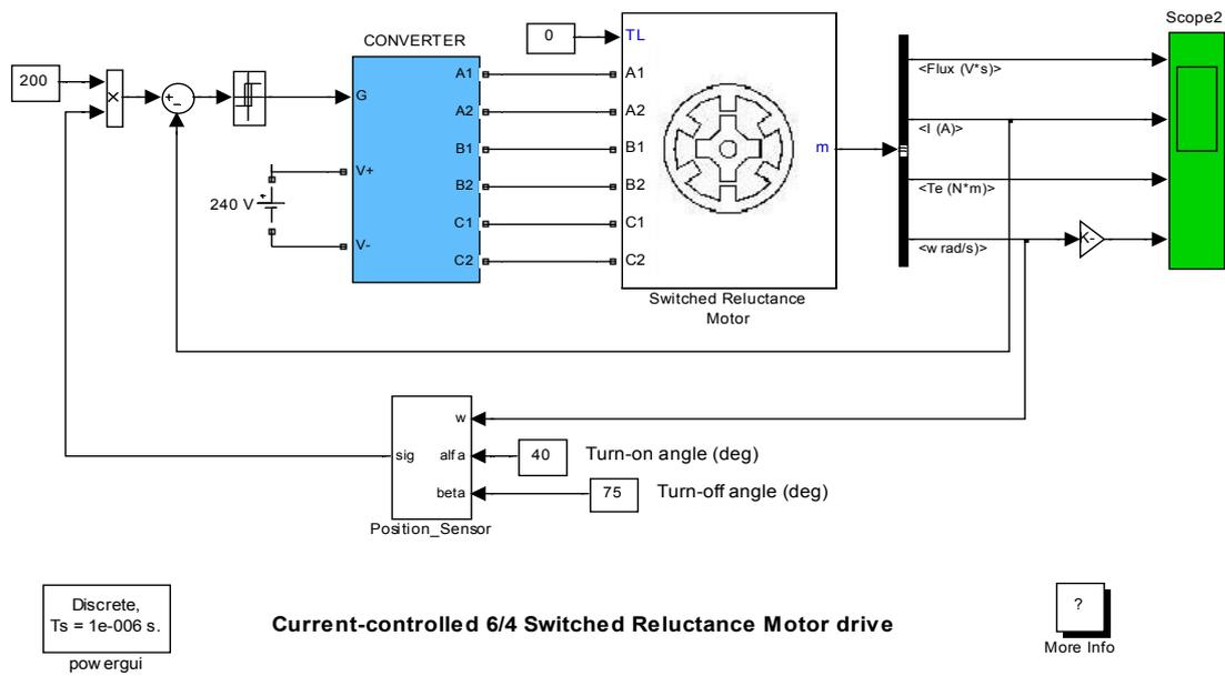
Fig. 7 Simulink model of 6/4, Switched Reluctance Motor
