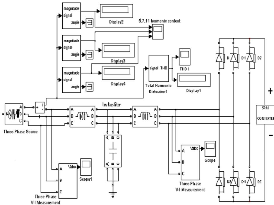
Fig. 9 Simulink Model of Converter Control strategy
