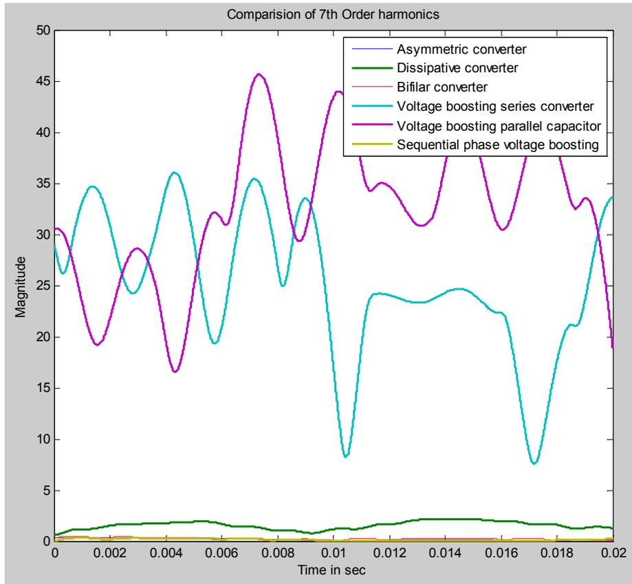
Fig. 23 7<sup>th</sup> Order Harmonics with Star Delta + Low Pass Filter
