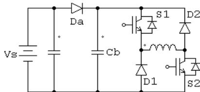
Fig. 4 Voltage Boosting Converter (Parallel Capacitor)
