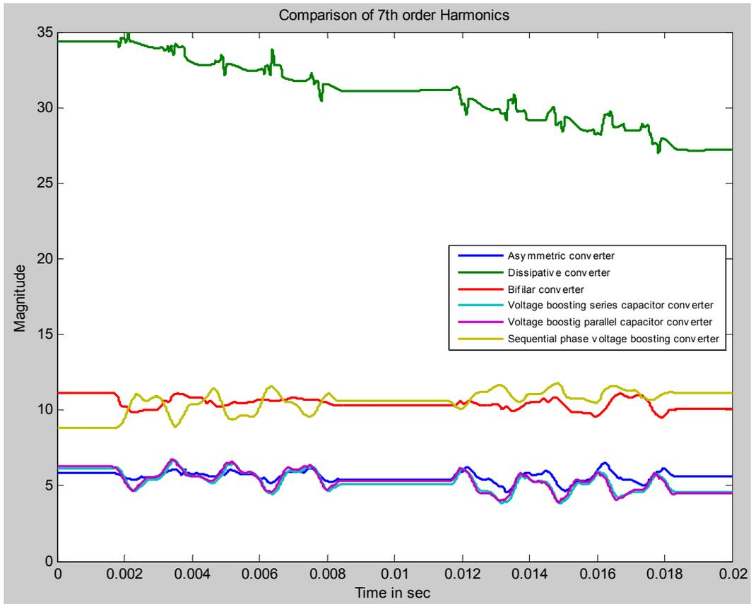
Fig. 11 7<sup>th</sup> Order Harmonics without Harmonic Reduction Techniques
