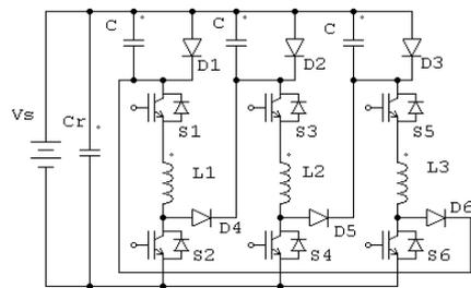
Fig. 6 Sequential Boost Converter
