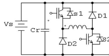
Fig. 1 Asymmetric Converter
