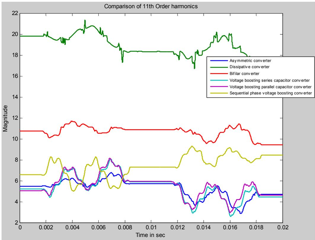
Fig. 12 11<sup>th</sup> Order Harmonics without Harmonic Reduction Techniques
