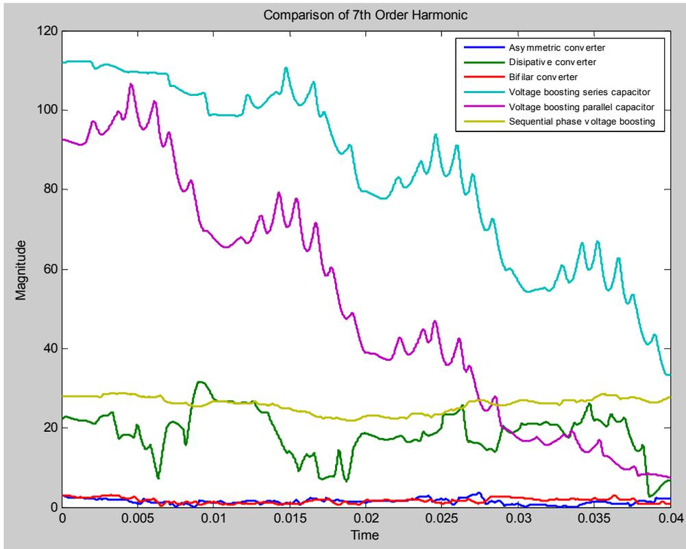
Fig. 15 7<sup>th</sup> Order Harmonics with Star Delta Transformer
