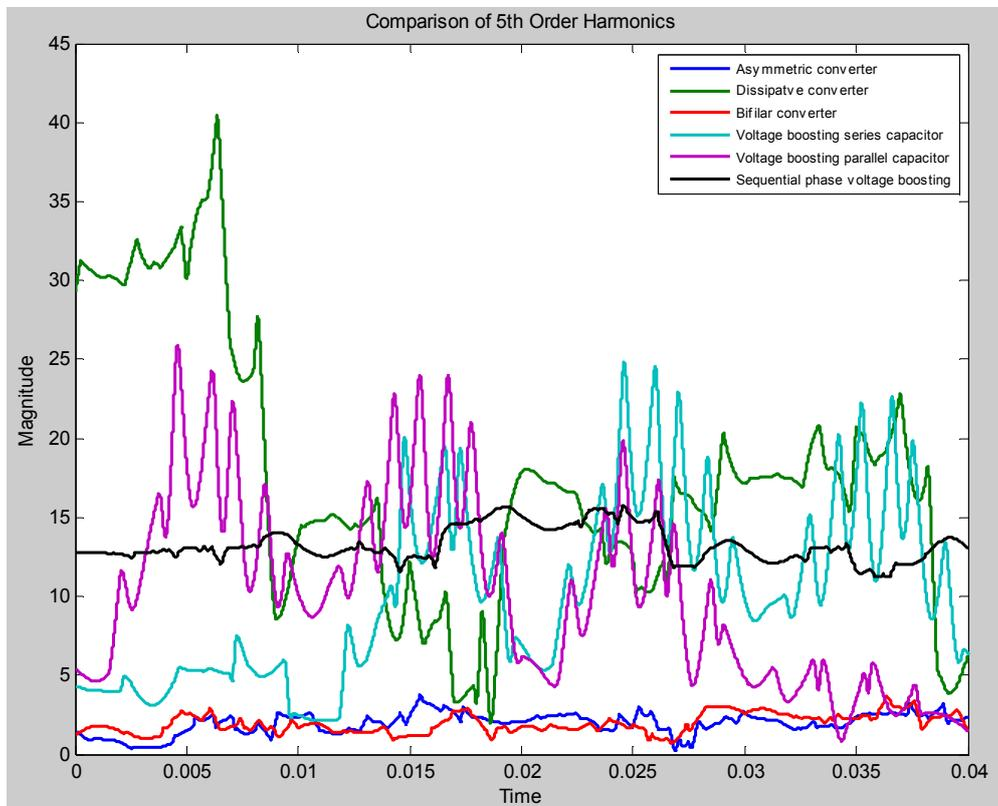
Fig. 14 5<sup>th</sup> Order Harmonics with Star Delta Transformer
