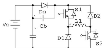
Fig. 5 Voltage Boosting Converter (Series Capacitor)
