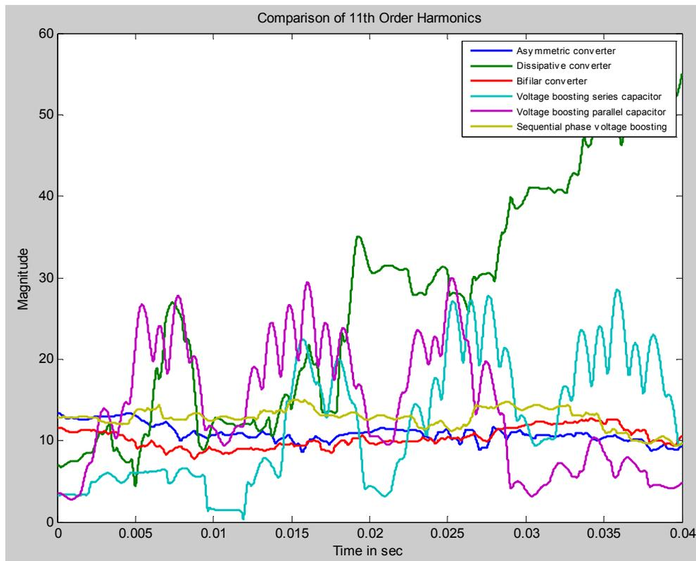
Fig. 16 11<sup>th</sup> Order Harmonics with Star Delta Transformer
