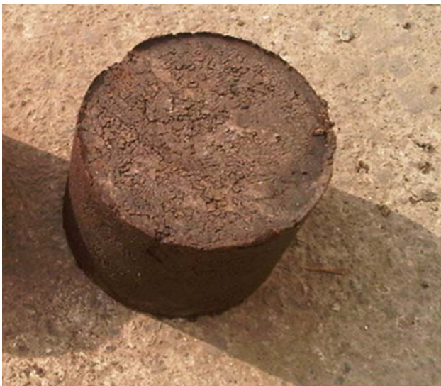
Fig. 1 Molded nylon solution-stabilized soil
