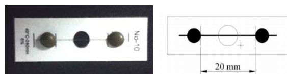
(a) Kenaf bast fiber test frame (b) Specimen dimension schematic diagram
