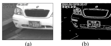
Fig. 2 Preprocessing, (a) Gray image from color input image, (b) Edge image from (a)
