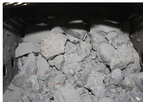
Fig. 3 Explosive spalling at 425°C on N series
