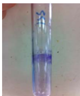
Fig. 2 Z. mobilis TISTR 551 Biofilm Formations on The Polystyrene Surface After 4 Days Cultivation. The Bacterial Attachment was Stained with Crystal Violet
