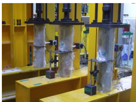
Fig. 4 Creep test of base course mixes
