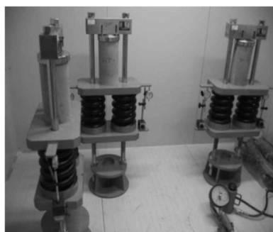
Fig. 2 Hydraulic creep test device
