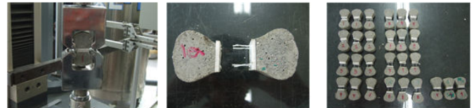
Fig. 8 JCI SF-8 dog-bone test of specimens
