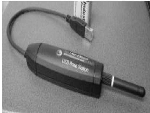
Fig. 3 Wireless Radio Frequency Basestation
