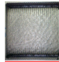
Fig. 4 Sample pocket milled surface
