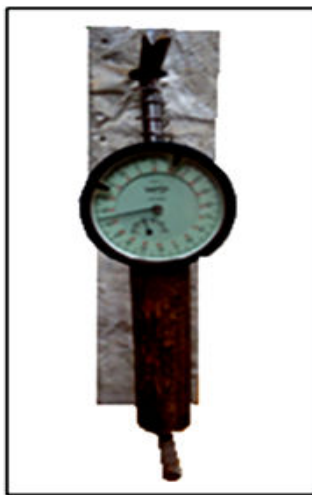
Fig. 4 Disposition of test pieces when testing shrinkage
