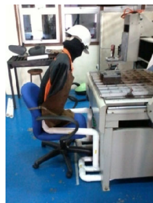
Fig. 2 Dummy welder in sitting position
