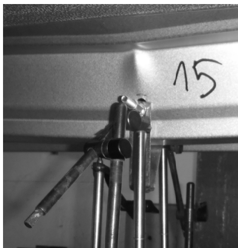
Fig. 12 End of testing of second phase (local buckling)
