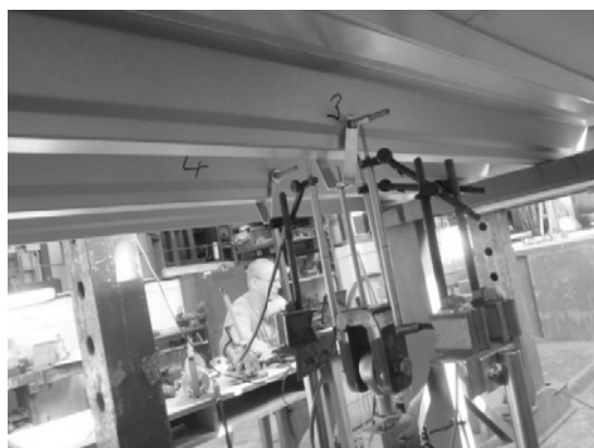
Fig. 7 Anchoring system with “V” clamp and tensile hydraulic cylinder
