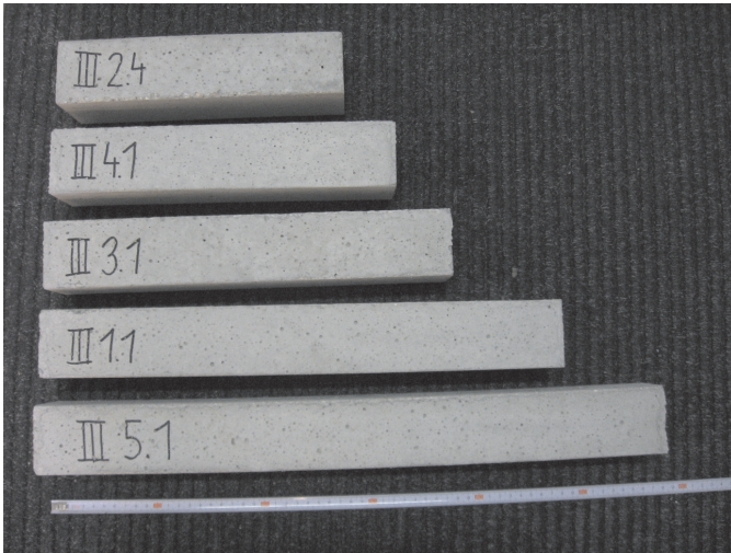
Fig. 7. Five different lengths of concrete samples.
