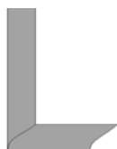
Fig. 8 Initial imperfection of the beam (bottom flange, from below)
