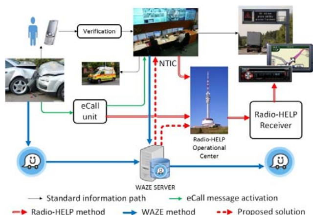
Fig. 1 Transmission and acquisition of information in the event of an accident with the use of eCall, Radio Help and WAZE (Author)
