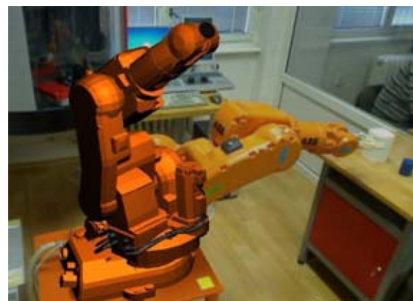
Fig. 4 Virtual model of robot in real environment
