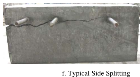
f. Typical Side Splitting
