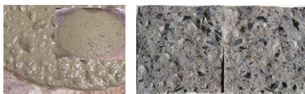
Fig. 5 SCC Behavior showing no sign of Segregation
