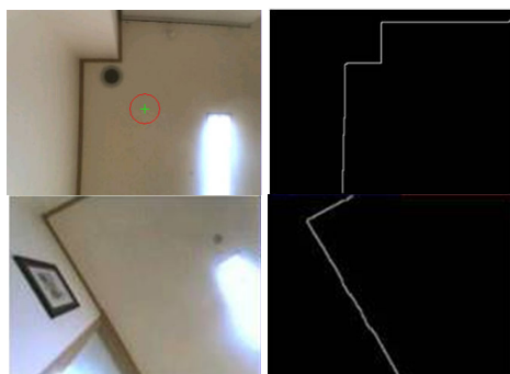
Fig. 4 Line and corner features in the local spaces
