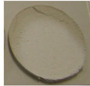
Fig. 5 Underside of the delaminated coating from sample TC1600
