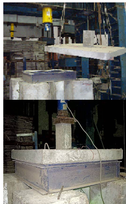
Fig. 2 General view of flat slabs and Test set up
