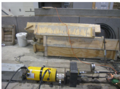
Fig. 4 Pullout test setup and strand gripping
