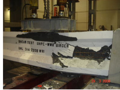
Fig. 8 Girder test (limit state)
