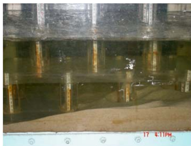
Fig. 12 Maximum scour depths at piers and combined piles after 24 hour
