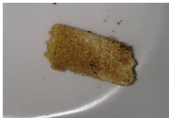
Fig. 9 Sintering of composite catalyst bed after test
