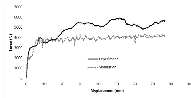
Fig. 5 Comparison experimental and numerical of force-displacement curves of a tube on 15° angled die ( \mu is constant=0.25)
