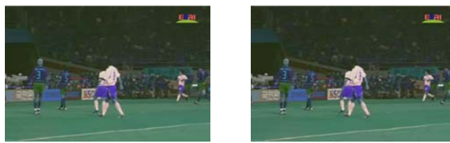
(a) Fixed QP (PSNR 35.55dB) (b) Proposed (PSNR 35.91dB)
