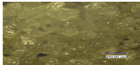
Fig.1 The morphology of resin coated sand
