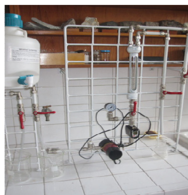
Fig. 5 Installation with vertical reactor to filter emulsions
