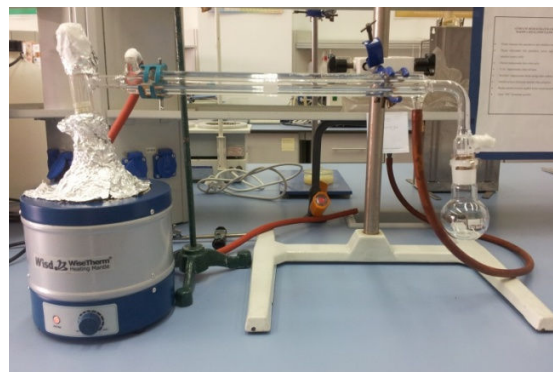
Fig. 7 Conventional distillation process
