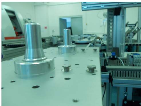
Fig. 11 Final product of Penholder in system iCIM 3000
