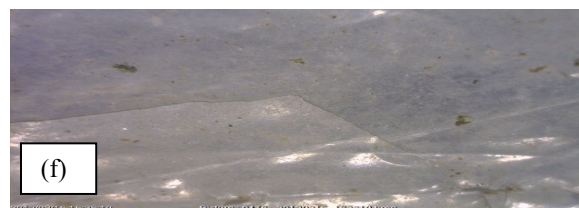
Fig. 4 (a) Control sample (b) Exposed 1 st month. (c) Exposed 2 nd month (d) Exposed 3 rd month. (e) Rougher surface at 4 th month exposure (f) Fragmenting started in sample at 5 th month
