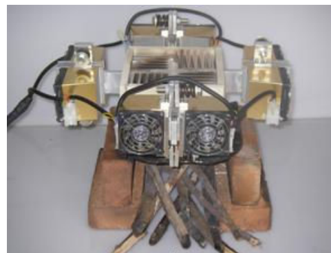
Fig. 12 To gen. the power with dead wood
