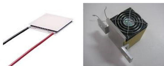
Fig. 7 TE (left) and cold sink (right)
