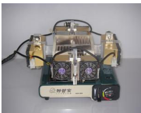
Fig. 11 To gen. the power with portable gas stove
