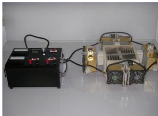
Fig. 8 The thermoelectric power generator system
