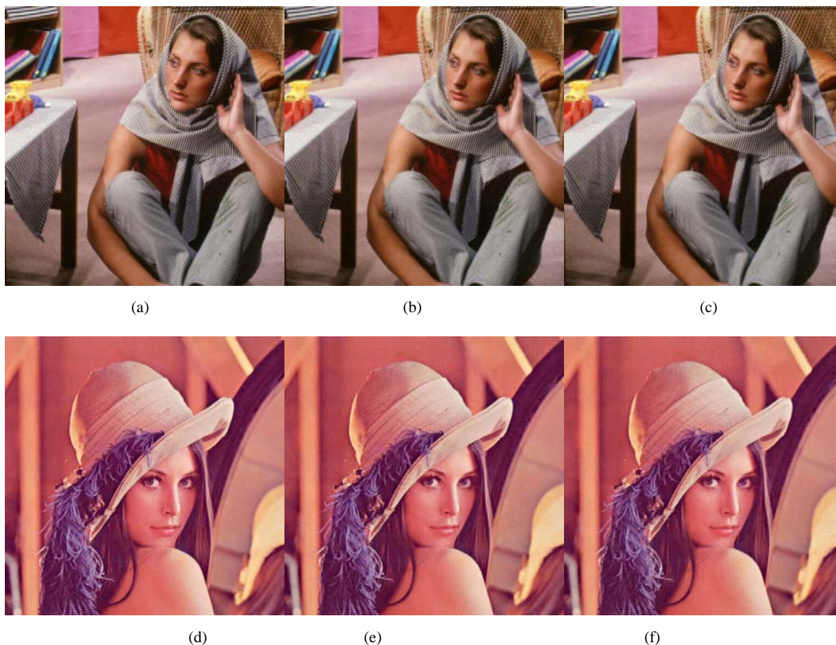
Fig. 3 Coding results of “Barbara” and “Lena” color images at visually lossless quality. (a) original “Barbara” color image, (b) coding “Barbara” color image (bit rate=0.41) by using the conventional JPEG coder, (c) coding “Barbara” color image (bit rate=0.29) by using the JPEG coder with the perceptually tuned preprocessor, (d) original “Lena” color image, (e) coding “Lena” color image (bit rate=0.36) by using the conventional JPEG coder, and (f) coding “Lena” color image (bit rate=0.24) by using the JPEG coder with the perceptually tuned preprocessor
