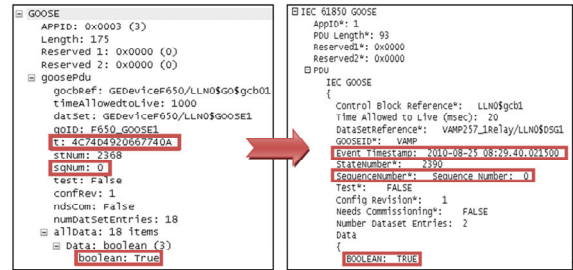
Fig. 15 GOOSE performance test – Wireshark (left) vs. Ethereal analyzer (right)
