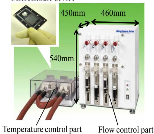
Fig. 1 Laboratory microfluidic device system
