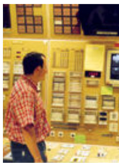
Fig. 4 Hybrid simulator developed by GSE Systems for nuclear reactor control rooms: the three boards are scale 1 on-touch screens and all components are virtual
