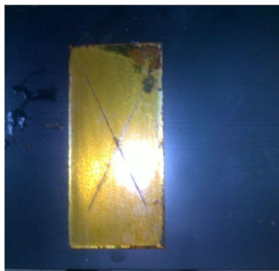
Fig. 6 Salt spray resistance of PU5 after 950 hours
