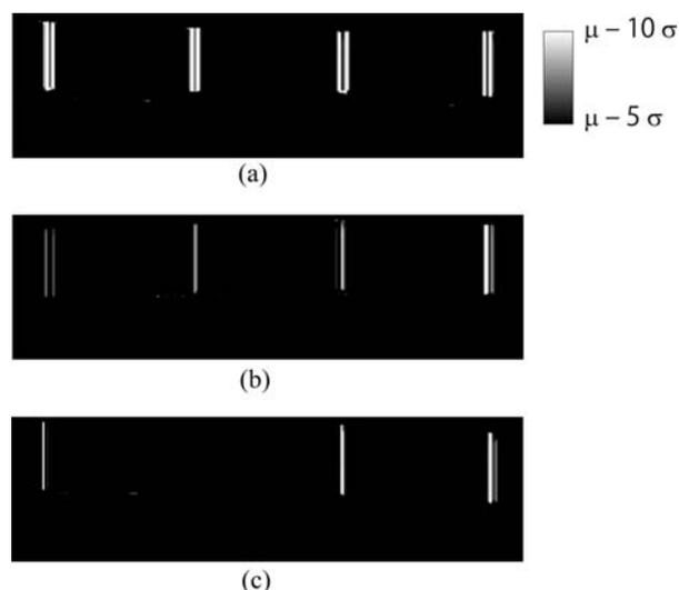
Fig. 3 Normalized cross-correlation profiles of three ROIs with four wires (a) 0.2, (b) 0.1, and (c) 0.05 mm in diameter. The size of each ROI is 1 x 3.5 cm.  $\mu$  and  $\sigma$  are the average and the standard deviation of the top 90% of the correlation coefficients in each ROI.
