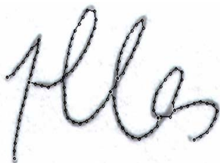
Fig. 2 strokes of a signature: extracted points (black) and end points of the strokes (white)
