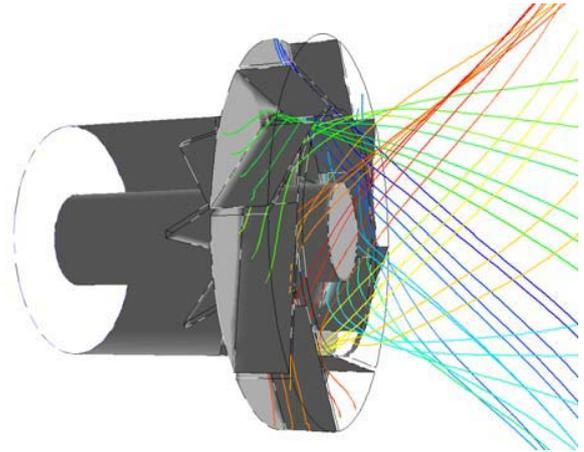
Fig. 3 Tangential flow pathlines passing through the tangential
