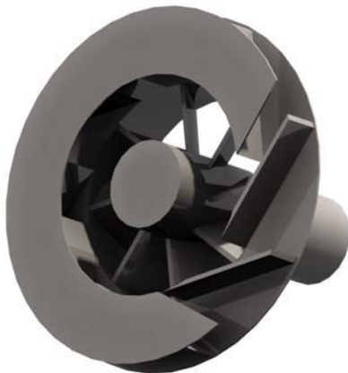
Fig.1 The concept of the new swirler with a cutout in the outer shroud showing two of the tangential vanes
