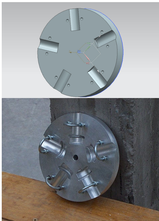
Fig. 5 A 0.34m hub diameter for a propeller fan
