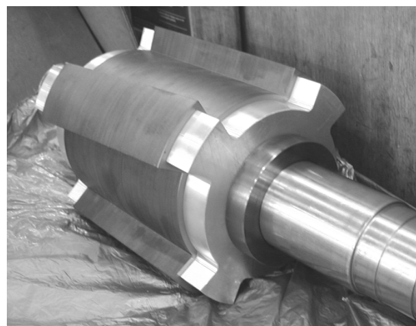
Fig. 14 Skewed rotor of 6-phase RDCM
