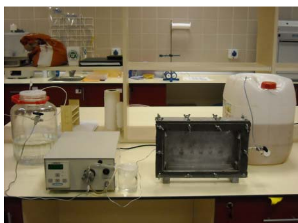
Fig. 3 2-D flow-cell experimental setup
