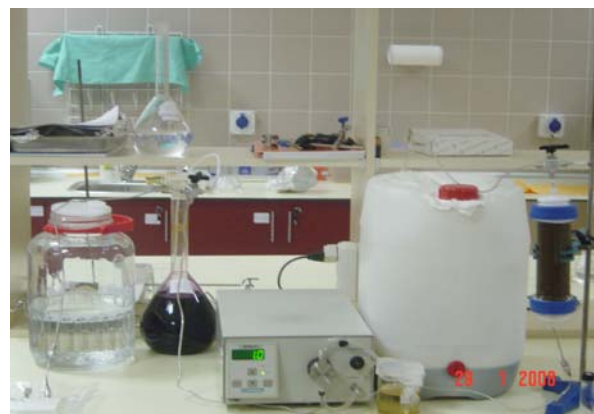
Fig. 2 1-D flow-cell experimental setup
