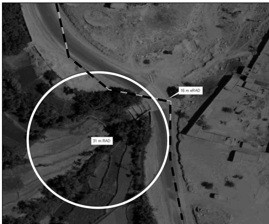
Fig. 17 Comparison of measured ROC (RAD) and the calculated effective ROC (eRAD) for a sharp curve
